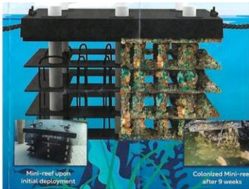
Mini Reefs are tested for durability and are created with marine grade materials. Mini Reefs have been shown to have an estimated 500-year lifespan and filter 30,000 gallons of water per day. They are akin to 'nature's kidneys' as they attract bivalves that clean the water while creating oxygen, and they provide a habitat for juvenile sea life. Once established, scientists report reefs will support some 300 fish and 200 crabs per year.
